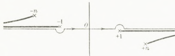
FIGURE 9. Singularities and branch-cuts in the complex \lambda -plane on the present method.
